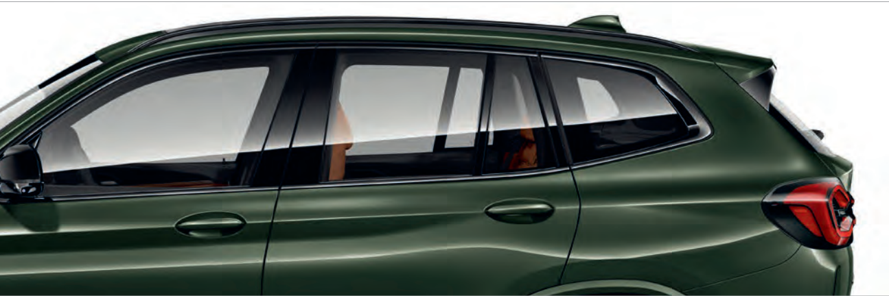
□ The M high-gloss Shadow Line includes numerous equipment details in Black high-gloss: side frame trim strips, window recess finishers, exterior mirror caps, mirror base and triangle, B-pillar trim panels and window guide bars on the rear doors.
