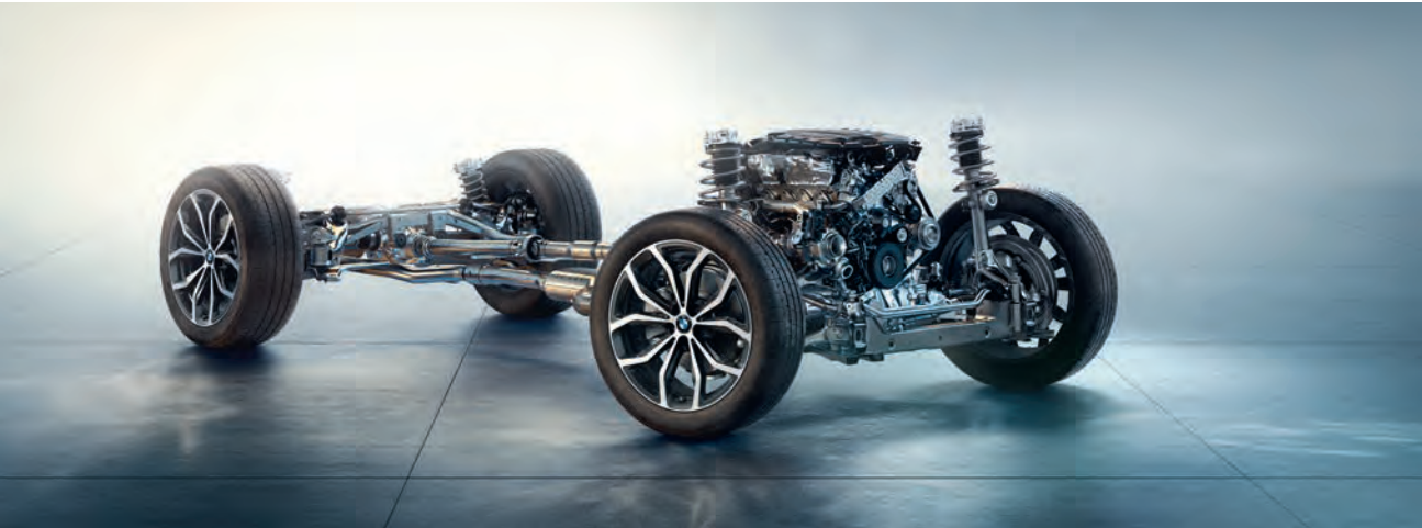
□ The adaptive suspension makes it possible to ideally adjust the damper characteristics to suit any given driving situation, improving roll comfort and driving dynamics. In addition to the standard COMFORT setting for increased driving comfort, the SPORT program can also be selected for athletic damper settings.
