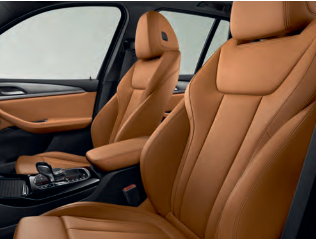
■ The adjustable Sport seats for the driver and front passenger feature numerous adjustment options, including fore-and-aft position, and the backrest and seat angle. Thanks to larger seat and backrest bolsters, and well-defined side bolsters, they provide excellent ergonomics and a high degree of lateral support.
